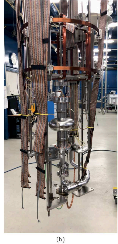
Figure 2: Technical drawing of the test cryostat in the AMTF at DESY with four cavities [10, p.6] (a), and image of insert 2 with one single-cell SRF cavity (b).
